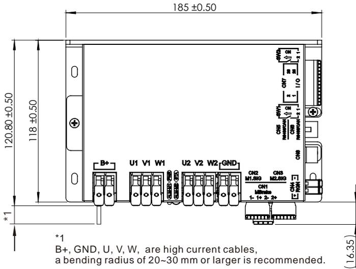
Recommended bending direction for the motor feedback signal wire
